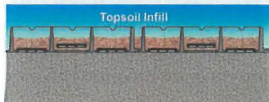
Figure 10. Sweep out topsoil infill
