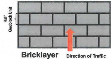
Figure 6 Bricklayer Laying Pattern
